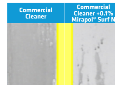
After 3 soiling cycles The surface is pre-treated once with the cleaner formulation and then soiled and rinsed several times
